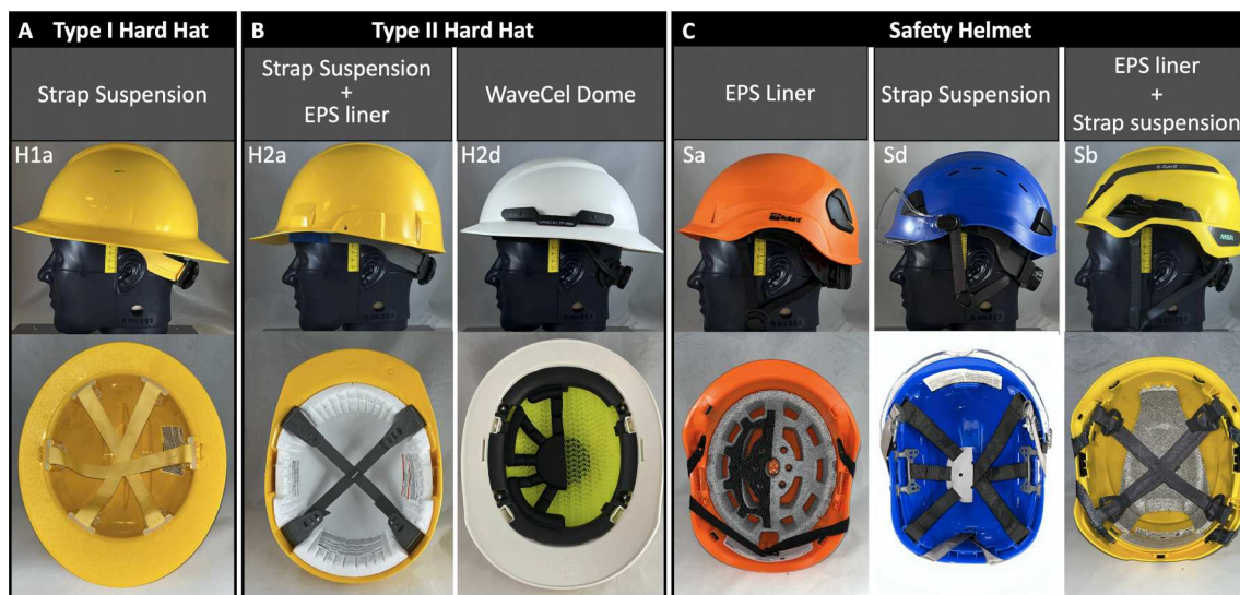
Fig. 1. Examples of helmet types in the three helmet categories: A) Type I hard hats had a strap suspension; B) Type II hard hats had a strap suspension combined with an EPS liner, or a cellular WaveCel dome; C) Safety helmets had either an EPS liner, or a strap suspension, or a combination of both. Images of the helmet inside are shown with the fit system and half of the comfort pad removed to better visualize strap suspensions and liners for impact mitigation.
