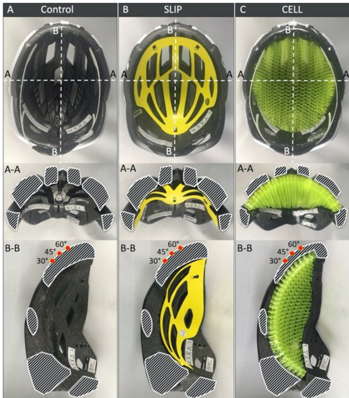
Fig. 1. Three helmet types with identical outer shell and liner thickness were tested: A) Standard EPS helmets (CONTROL); B) helmets with a MIPS slip liner for mitigation of rotational acceleration (SLIP); and C) helmets with a cellular structure for mitigation of linear and rotational acceleration (CELL). Sectioned EPS areas along transverse cut (A-A) and sagittal cut (B-B) are outlined in white for illustration. Impact locations corresponding to the 30°, 45°, and 60° anvils are denoted by red dots on sagittal cross-sections. (For interpretation of the references to colour in this figure legend, the reader is referred to the web version of this article).
